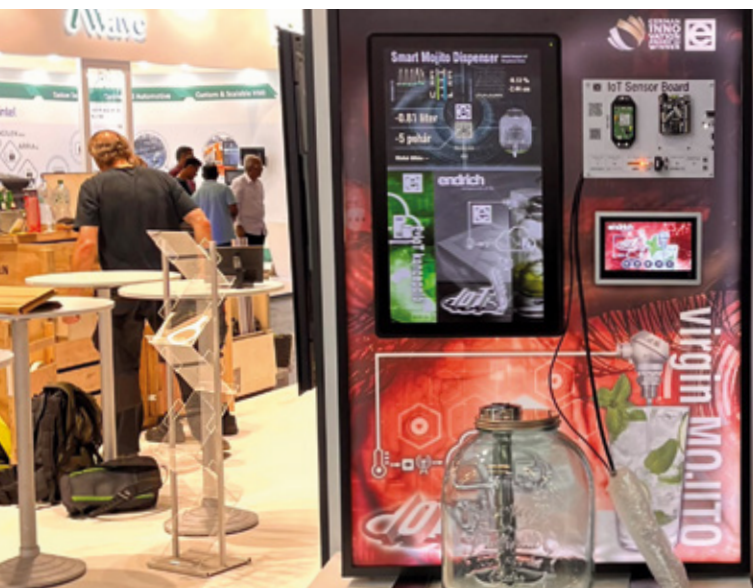
IoT Sensor Demo Board integrated in a Mojito Dispenser. Worldwide access to sensor data via the Endrich Cloud.
